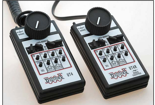
Two models are available. The UT4R adds radio wireless operation. (Digitrax Photo)
